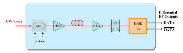
The integrated DPSK receiver combines a delay-line interferometer (DLI) with a balanced receiver to achieve compact size in a butterfly package. Compared with discrete components, the integrated receiver couples optical outputs from the DLI directly into the balanced photodetectors, resulting in smaller insertion loss and low channel skew, in addition to the elimination of fiber routing and matching.
